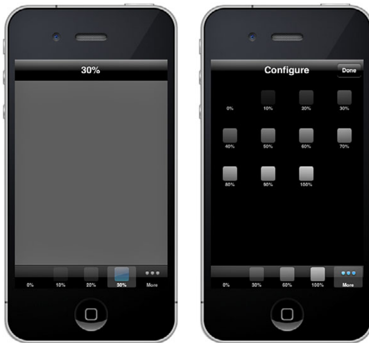
Figure 5-6 Tab bar controllers allow users to pick view controllers from a bar at the bottom of the screen (left side of the figure) and to customize the bar from a list of available view controllers (right side of the figure).
